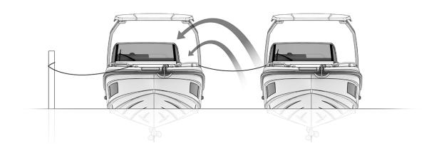
Figure 2.6 Running the engine in confined spaces
