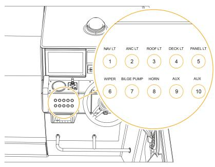
Figure 4.6 Controls on the function control panel
